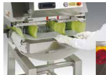
Tool free belt removal
