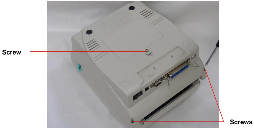
3. Remove 6 screws on **lower inner cover**.
